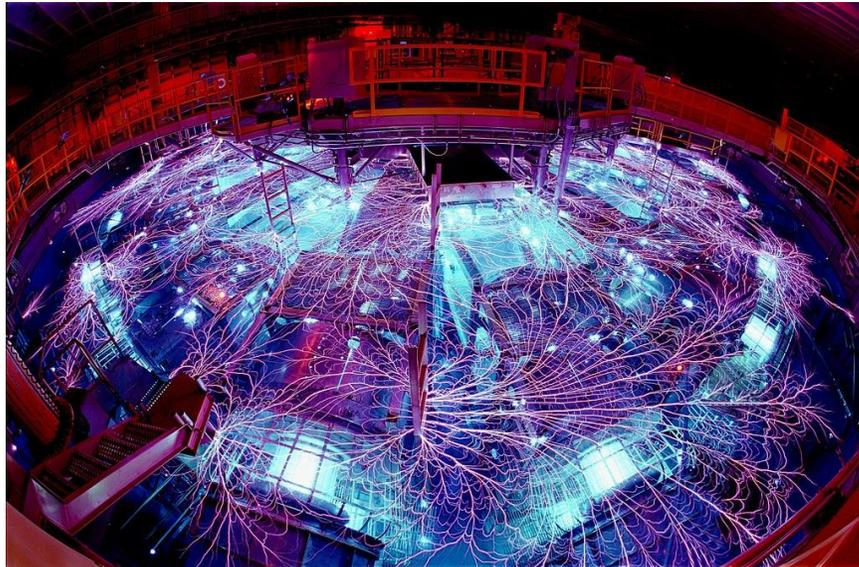
The Z machine compresses fusion fuel contained in a beryllium can (liner).
