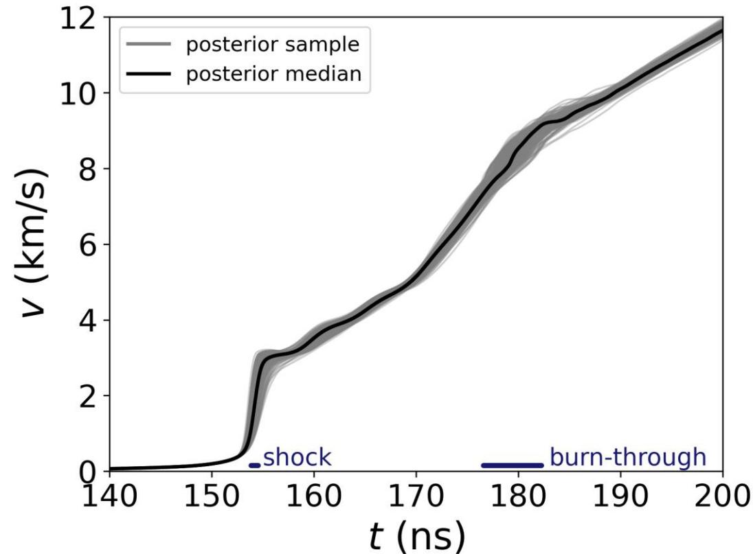
Current generated by the Z machine accelerates a piece of material outward; its velocity informs us of potential current losses.
