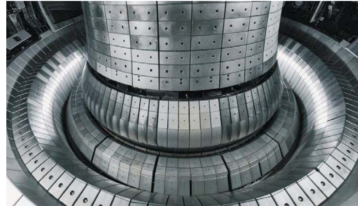
ASDEX in full tungsten configuration (Garching)
