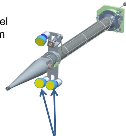
Radiochemistry collectors at 50 cm also house irradiated materials
