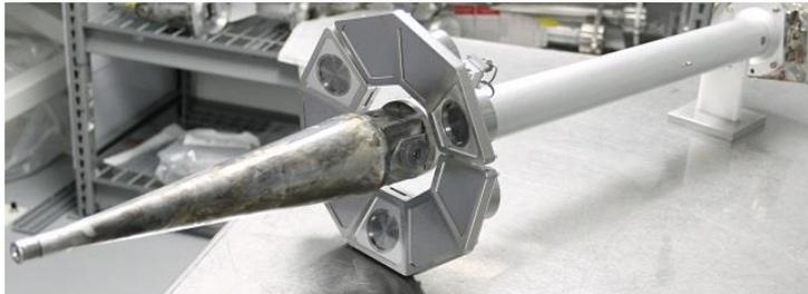
*Vast Area Detector for Experimental Radiochemistry (VADER), ~1% Solid debris collection*
