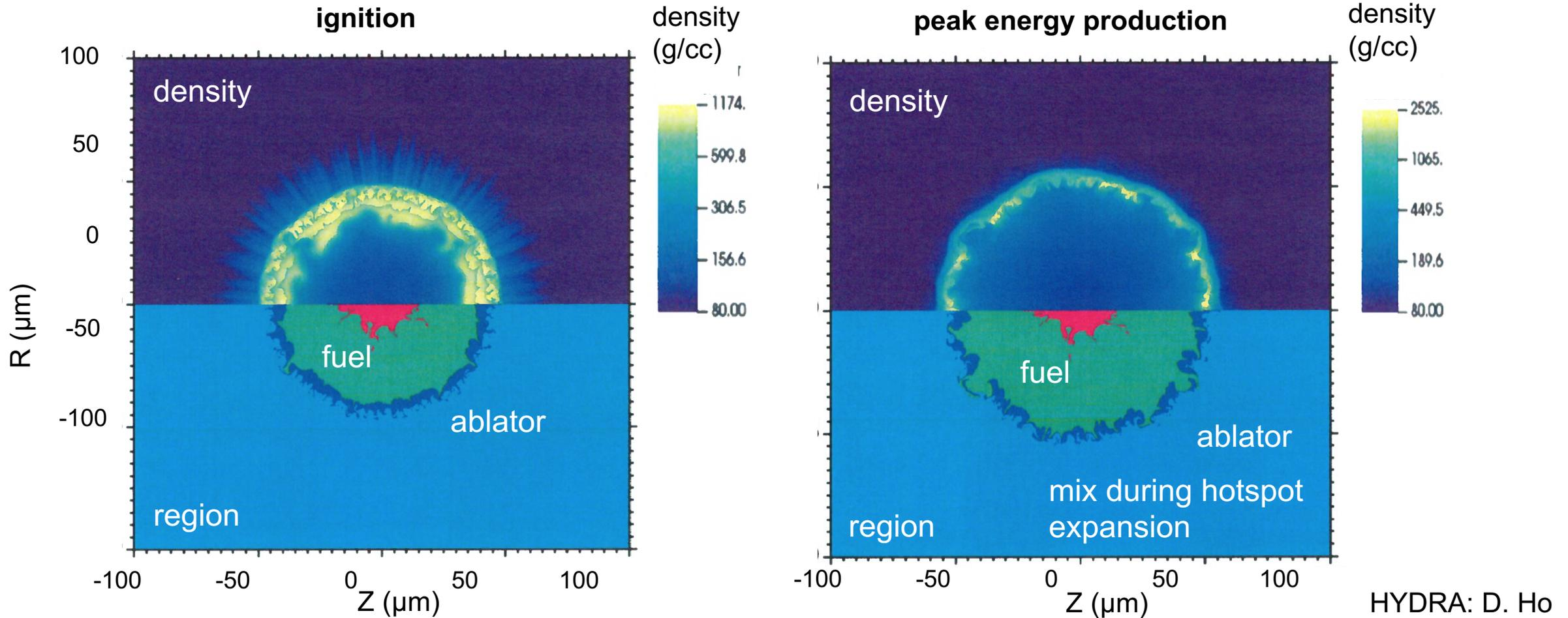
Good deceleration-stability results in an intact fuel ablator interface; the inner Be layer helps control expansion phase mix
