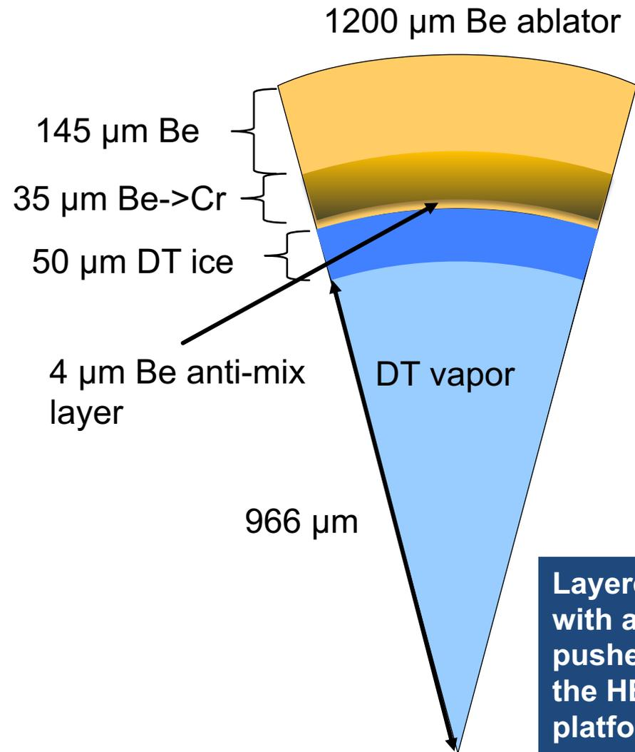
Layered design is optimized with a lighter, narrower peak pusher density region than the HED metal-gas mix platform
