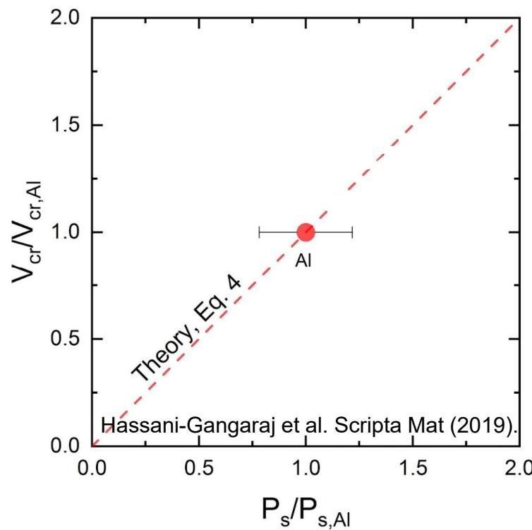
2. Pure metals isolate the **speed of sound** dependence
