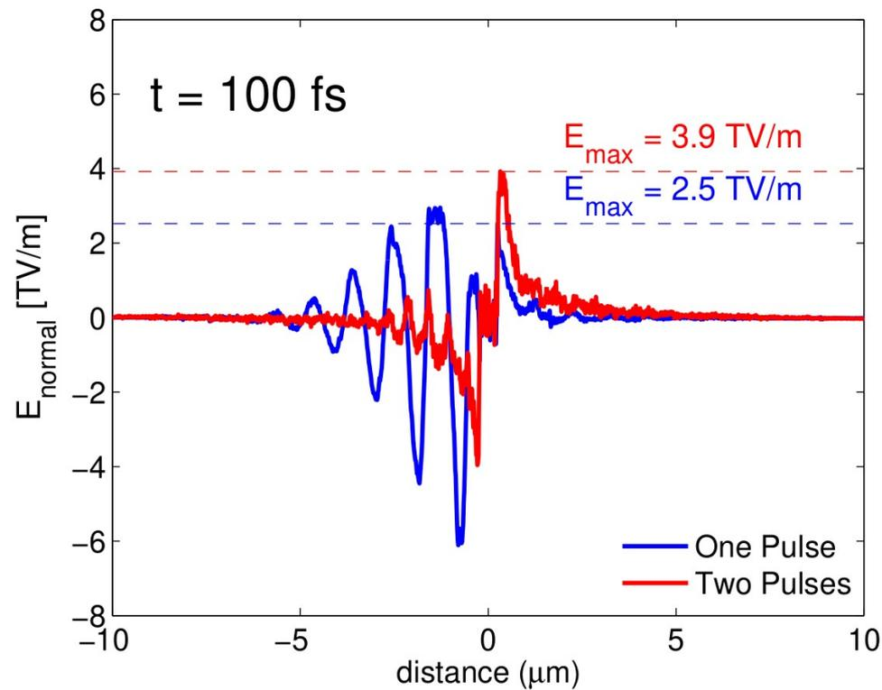
According to TNSA theory:  $E_{\max} \sim \frac{k_B T_{\text{hot}}}{e \lambda_D} \sim \sqrt{n_{\text{hot}} k_B T_{\text{hot}}}$
