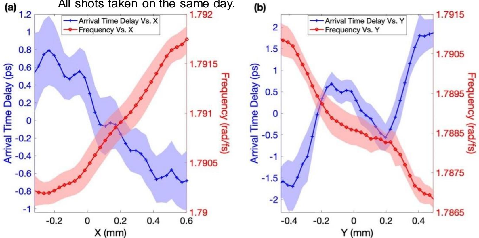
The phase curves provide these plots for pulse front tilt and spatial chirp for all shots, which corroborate the shear plots.
