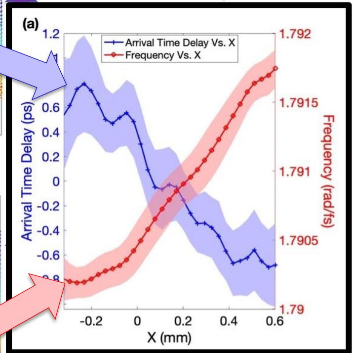
So, a change in slope of the linear phase across  $x$  means that the center frequency is moving across  $x$ .
