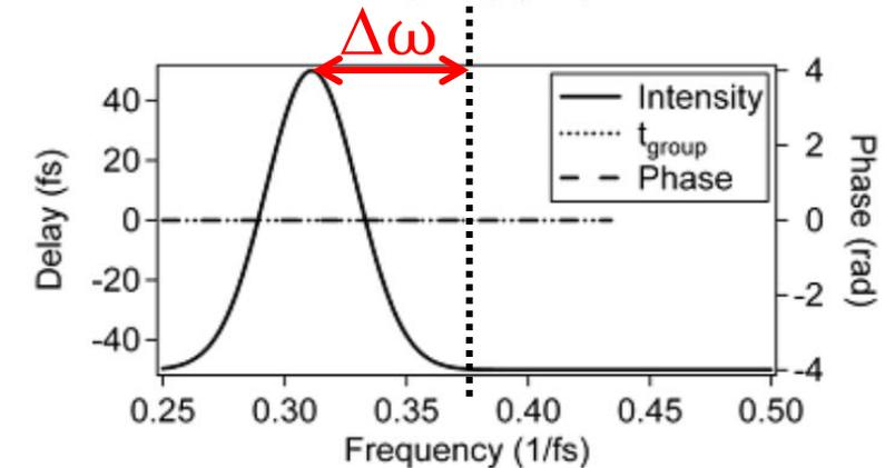
So, a change in slope of the linear temporal phase across  $x$  indicates that the center frequency is moving across  $x$ .
