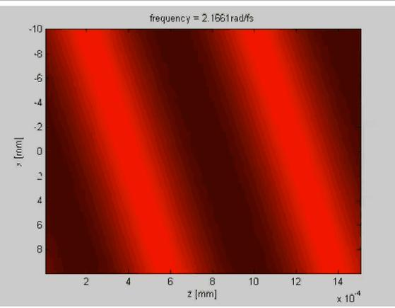
$$E(x, \omega) \propto \exp(R_{xx}x^2 + 2R_{x\omega}x\omega - R_{\omega\omega}\omega^2)$$
