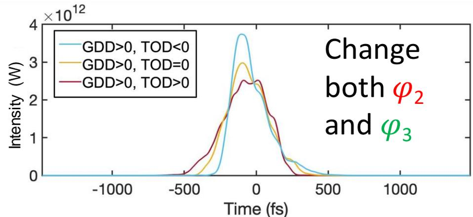
We can both accurately manipulate and measure the temporal pulse shape.
