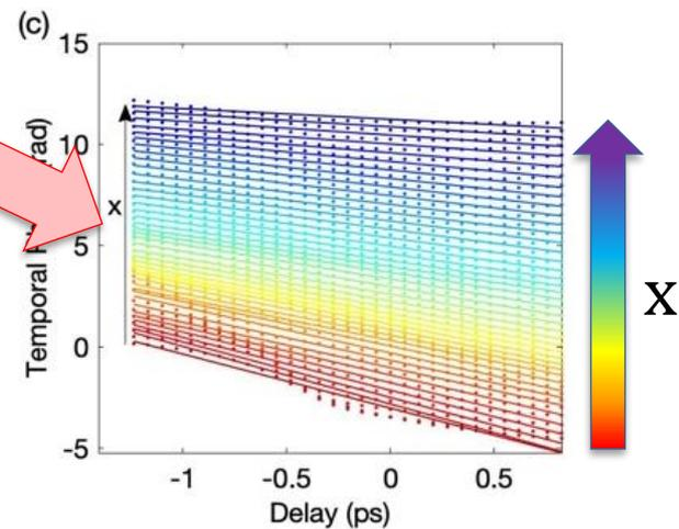
So, a change in slope of the linear phase across  $x$  means that the center frequency is moving across  $x$ .
