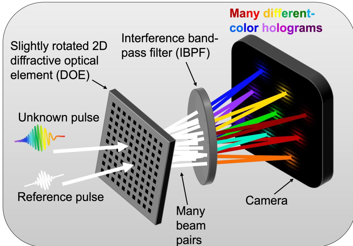
By spectrally resolving the holograms, we obtain the wavefront at each frequency present in the laser pulse.
