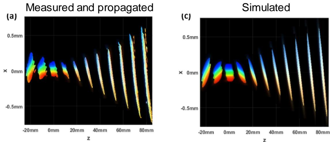
STRIPED FISH can also be used to obtain the electric field at the focus.
