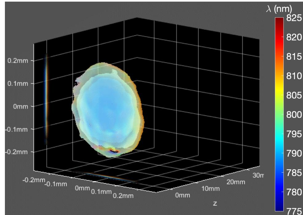
Measured ultrashort laser pulse with astigmatism and chirp.
