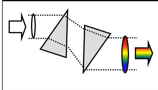
$$E(x, \omega) \propto \exp(R_{xx}x^2 + 2R_{x\omega}x\omega - R_{\omega\omega}\omega^2)$$
