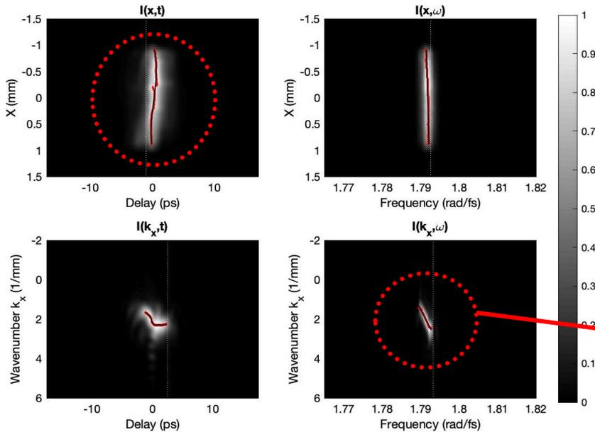
We tracked down the misalignment to the diffraction grating in the compressor and corrected the first-order alignment.
