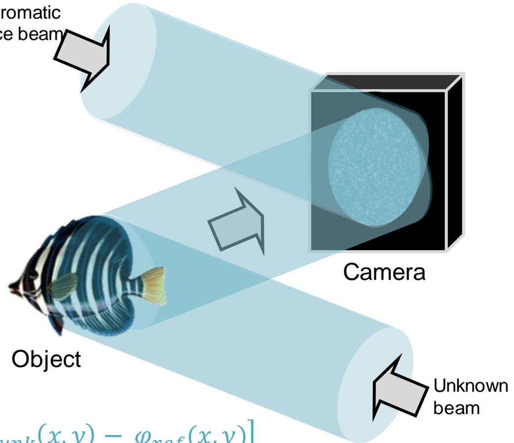
Holography can provide the wavefront of the laser pulse.
