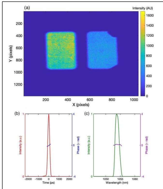
However, NIF-ARC's pulse could be spatiotemporally characterized by STRIPED FISH (simulated trace below).
