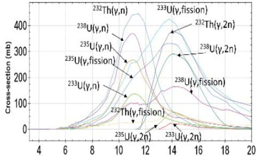
GDR cross-sections for  $(\gamma, n)$ ,  $(\gamma, 2n)$  and  $(\gamma, \text{fission})$  reactions span 8 – 20 MeV. Hence photo-neutron and photo-fission yields are highly sensitive to the gamma-ray fluence in this energy range.
