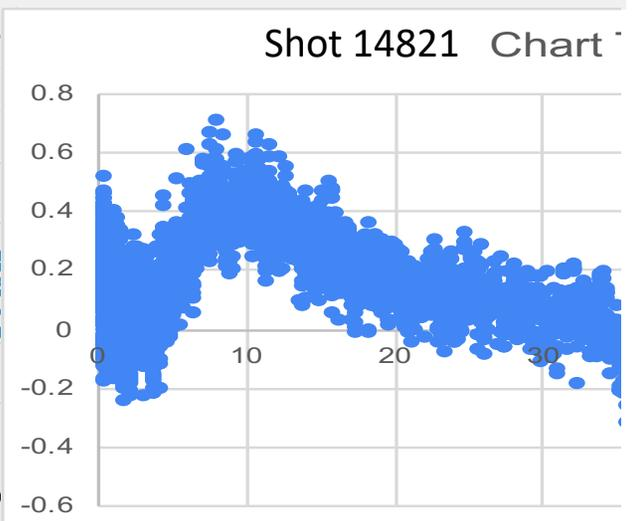
For very thick ( $\sim$  cm) targets,  $e^+e^-$  spectra almost identical, dominated by pairs created within  $\sim 1$  mfp of target back surface. Equal peak energies suggest that sheath fields did not affect the peak energy. Hence  $E_{\text{peak}}$  must come from gamma-ray spectrum
