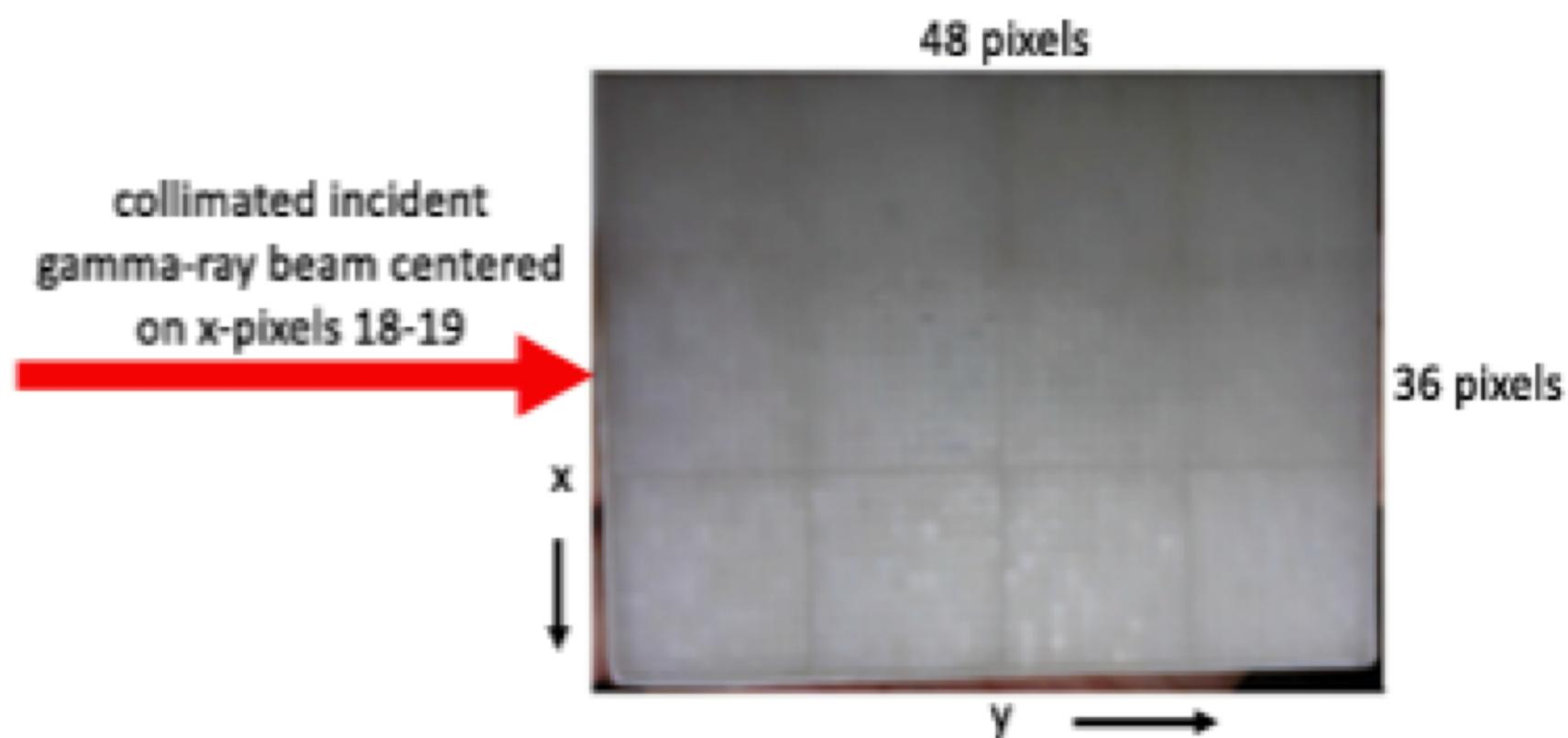
light patterns from different monoenergetic gamma-rays are clearly distinguishable
