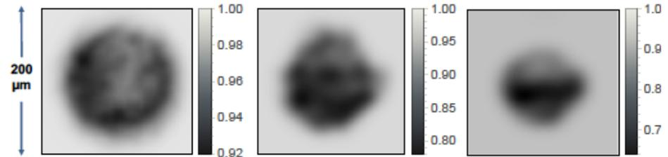
FIG.2. Compton radiographs of cryogenic THD layered implosion, recorded at BT-50ps, BT-10ps and BT+160ps.
