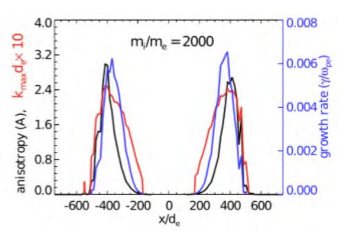
$$k_{\perp}^2 c^2 - \omega^2 - \sum_{\alpha} \omega_{p\alpha}^2 A_{\alpha} - \sum_{\alpha} \omega_{p\alpha}^2 (A_{\alpha} + 1) \xi_{\alpha} Z(\xi_{\alpha}) = 0$$
