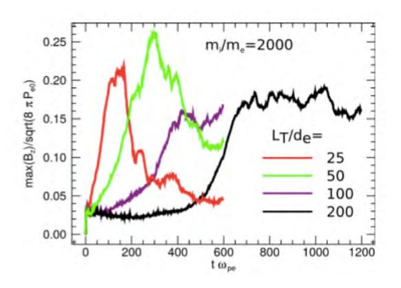
For small system sizes, magnetic field decays at late times due to ion-acoustic instability (predicted by Haines 97).
