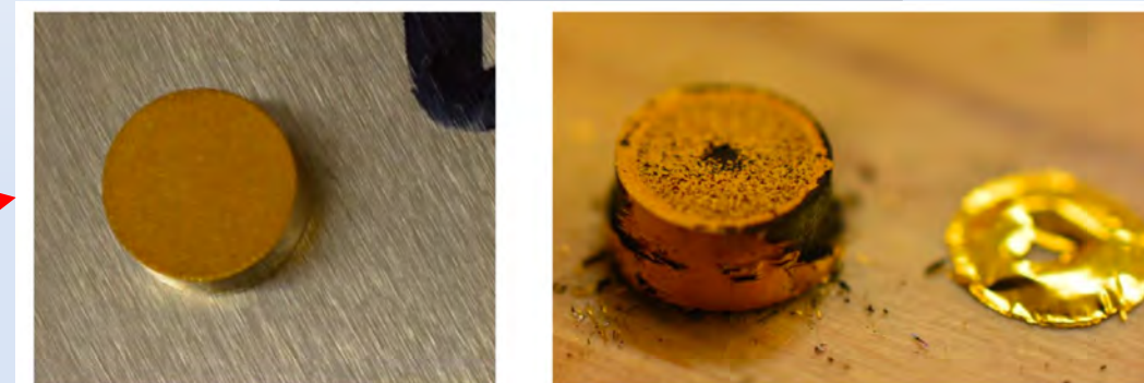
Gold-coated depleted uranium sample before (left) and after (right) ignition experiment.
